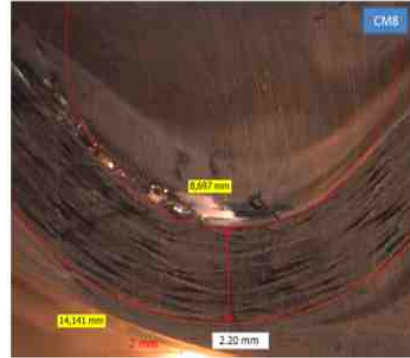
Figure 7b – Lower skin front spar radius
