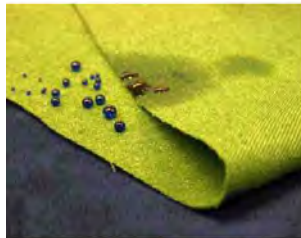
One side FC-finished fabric followed by one sided plasma treatment
