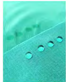
Two sided FC-finished fabric followed by one sided corona treatment
