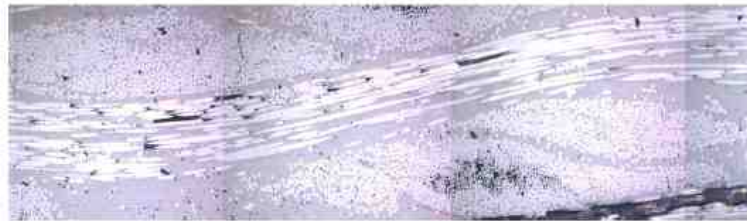
(a) Micrographic image of consolidated polypropylene (PP)/glass fiber commingled yarn composites
